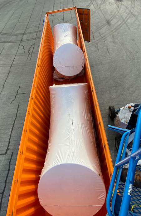
Pipe for LNG, approx 12,000lbs each.
